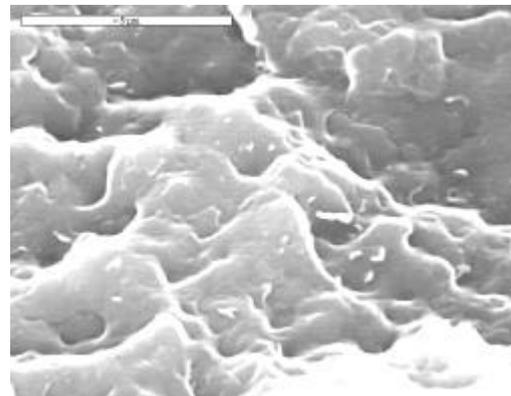
In SEM-Photo2 it can be seen that the nanoclay appearing as white particles on the polymer surface is very well dispersed. This is supported by the organic modification of the nanoclay and the two step compounding via a masterbatch.
